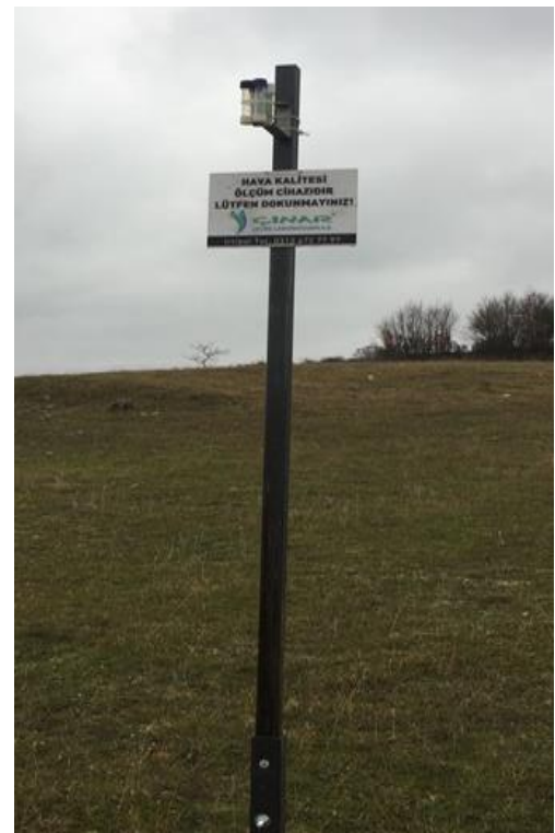
Air quality monitoring equipment used for monitoring dust in the Project area
