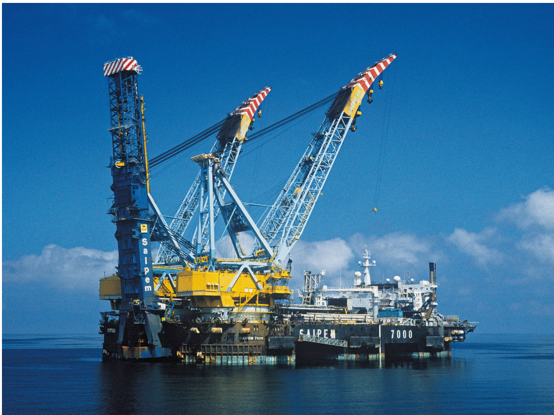
Figure 5.6 Typical Deep Water J-Lay Vessel
