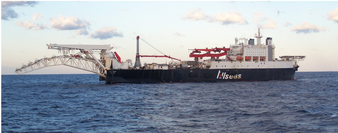
Figure 5.5 Typical Deep Water S-Lay Vessel
