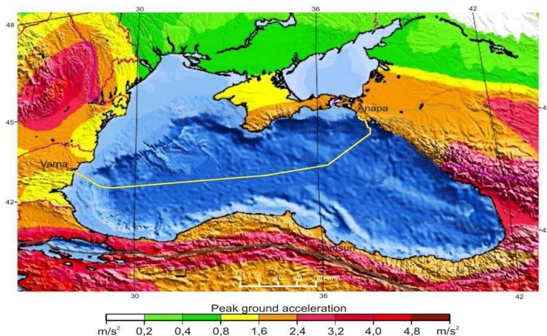
**Note:** the South Stream Offshore Pipeline is shown in yellow. **Source:** Ref. 7.17
