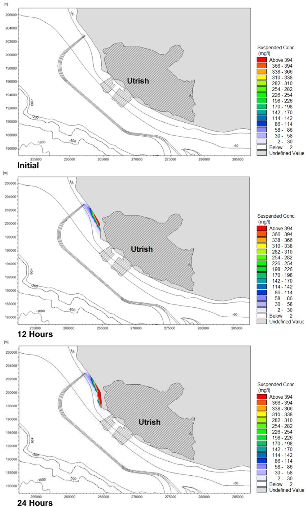
**Figure 3-3a Plume Development under Clockwise Currents (Scenario 1)**
