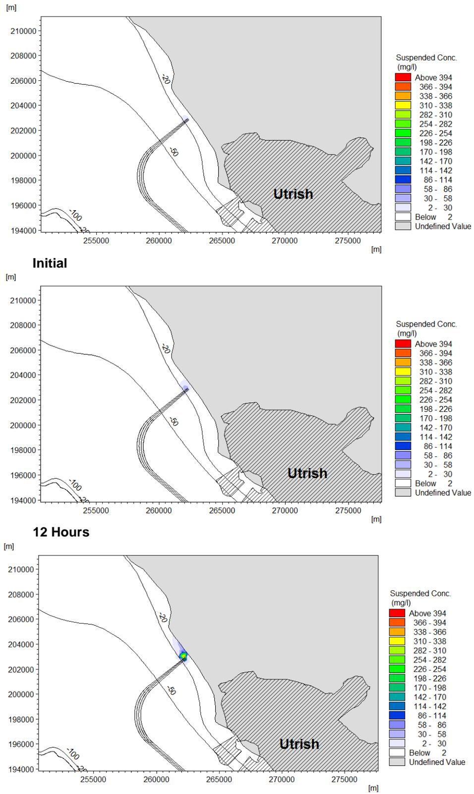
**Figure 3-4a Plume Development under Clockwise Currents (Scenario 2)**
