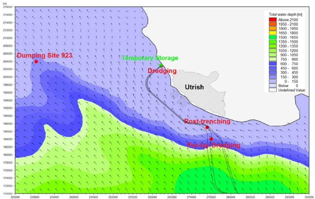
**Figure 3-2 Dredging and Disposal Locations (Counter-Clockwise Currents)**
