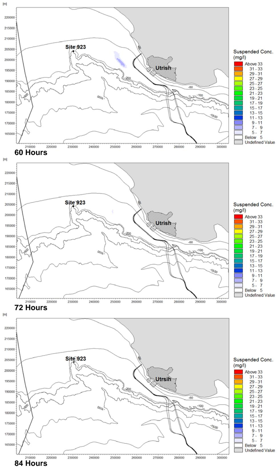
Figure 3-10b Plume Development under Counter-Clockwise Currents (Scenario 4)
