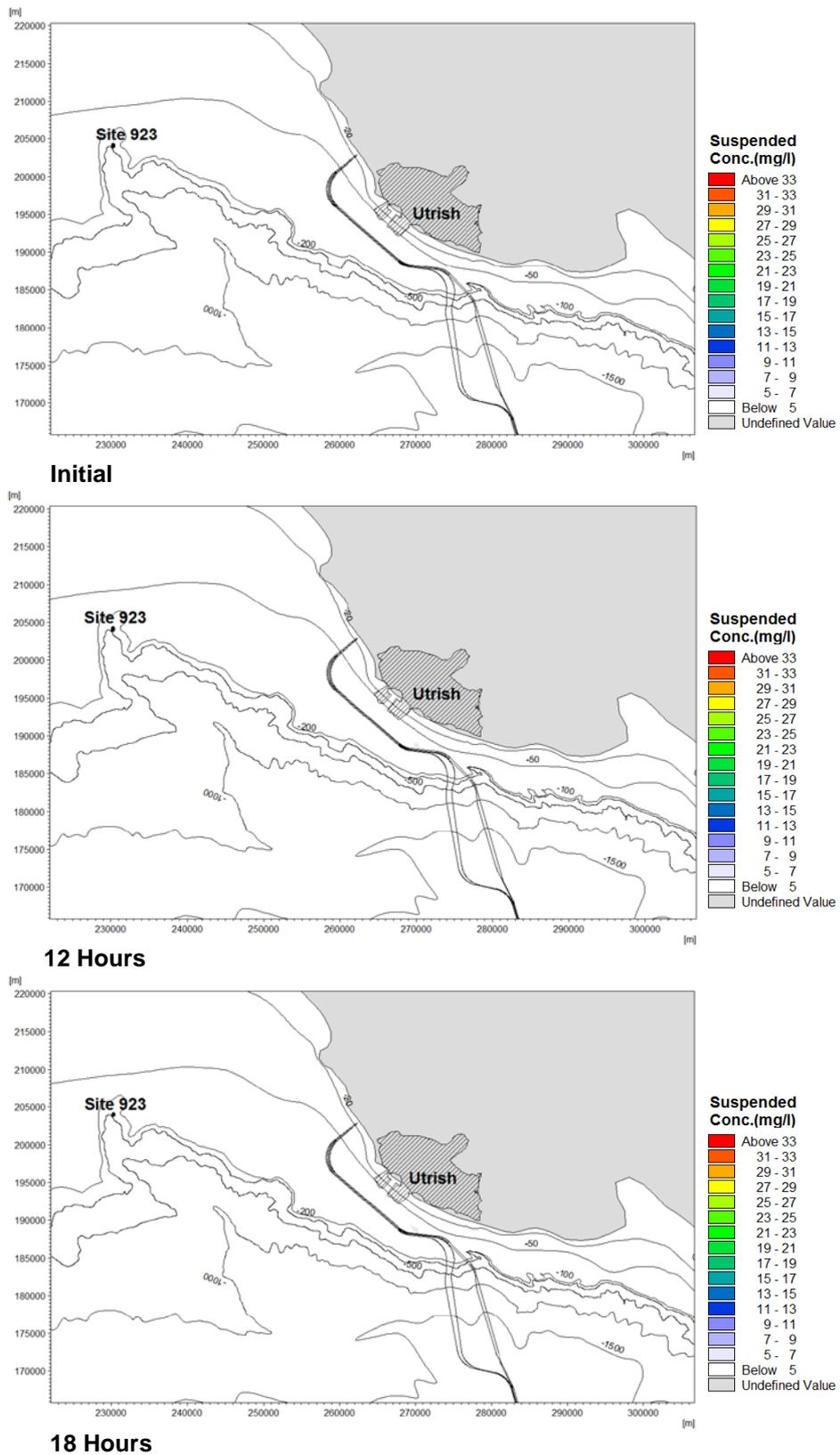
**Figure 3-20a Plume Development under Counter-Clockwise Currents (Scenario 6)**
