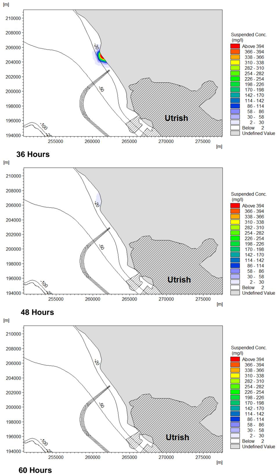
**Figure 3-4b Plume Development under Clockwise Currents (Scenario 2)**
