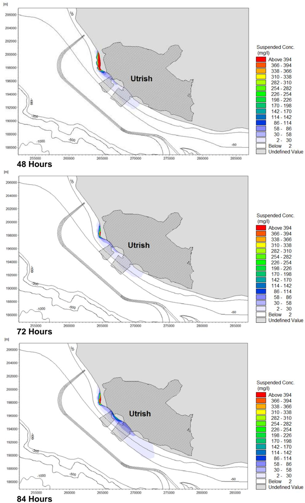
**Figure 3-3b Plume Development under Clockwise Currents (Scenario 1)**
