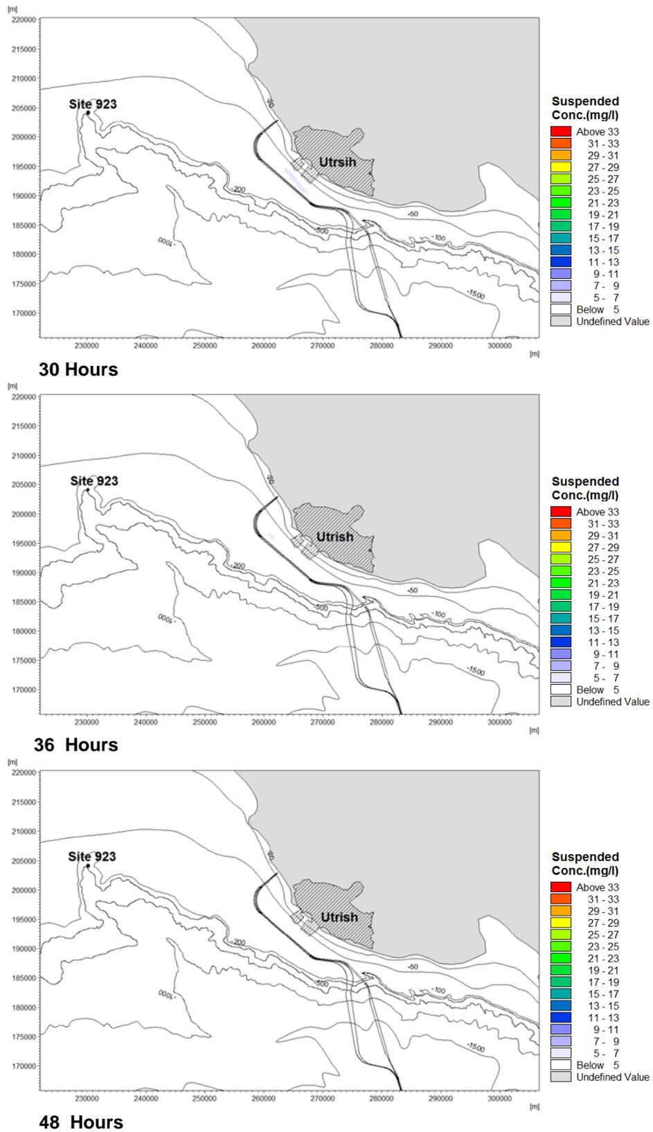
**Figure 3-20b Plume Development under Counter-Clockwise Currents (Scenario 6)**
