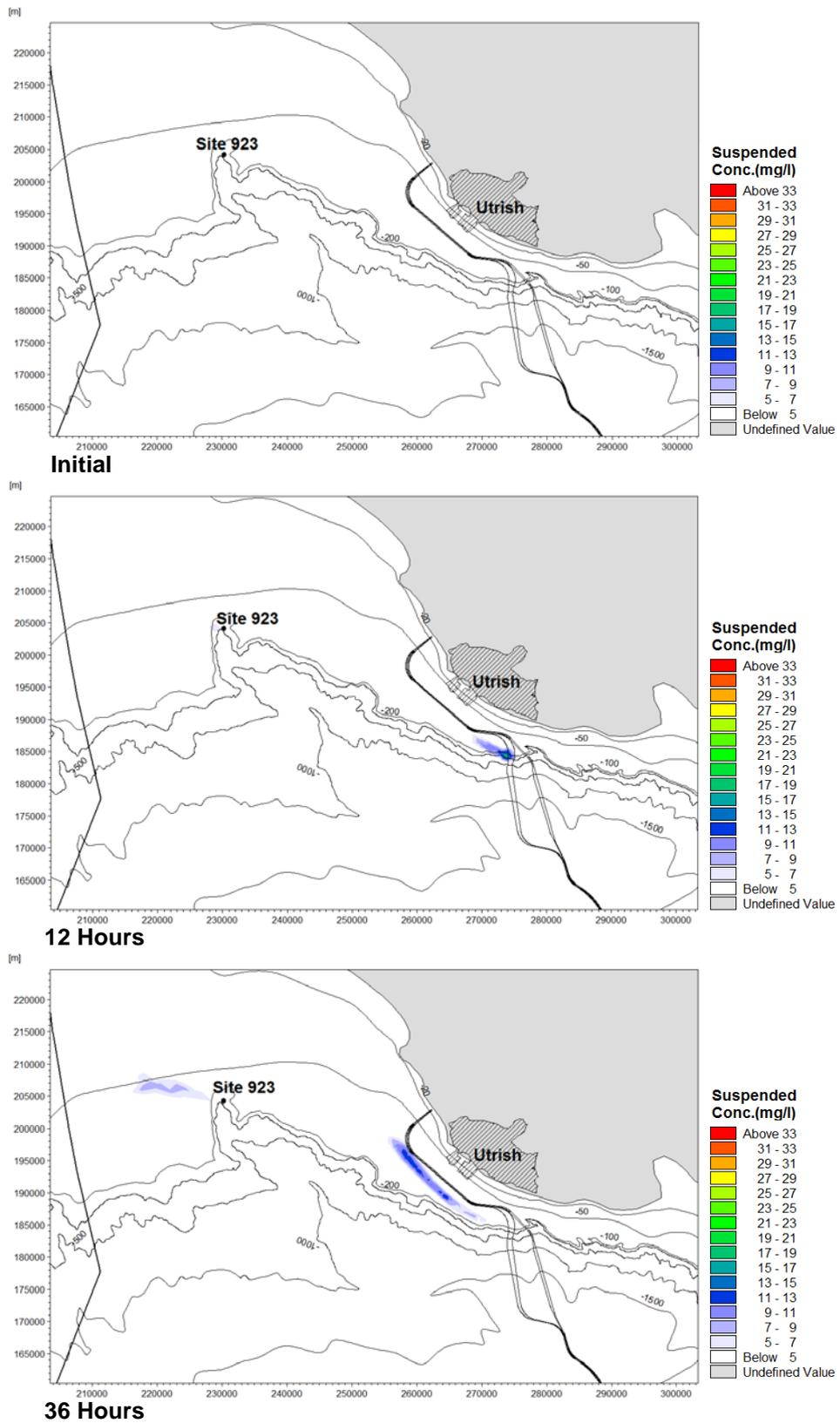
Figure 3-10a Plume Development under Counter-Clockwise Currents (Scenario 4)
