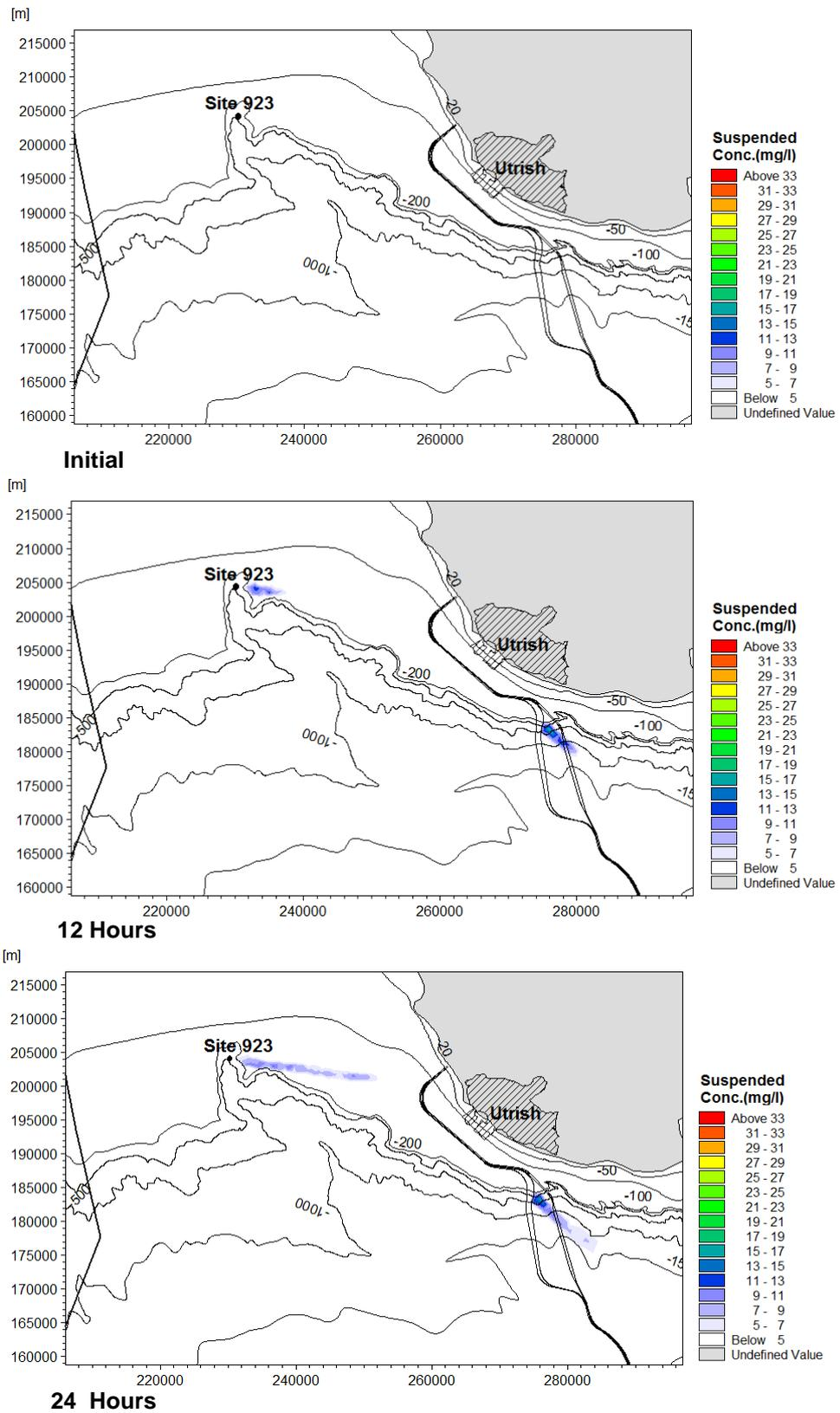
**Figure 3-9a Plume Development under Clockwise Currents (Scenario 3)**
