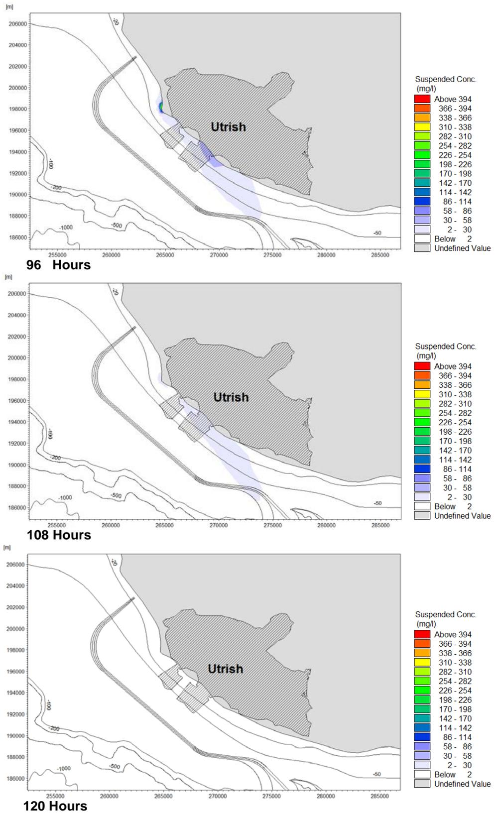
**Figure 3-3c Plume Development under Clockwise Currents (Scenario 1)**
