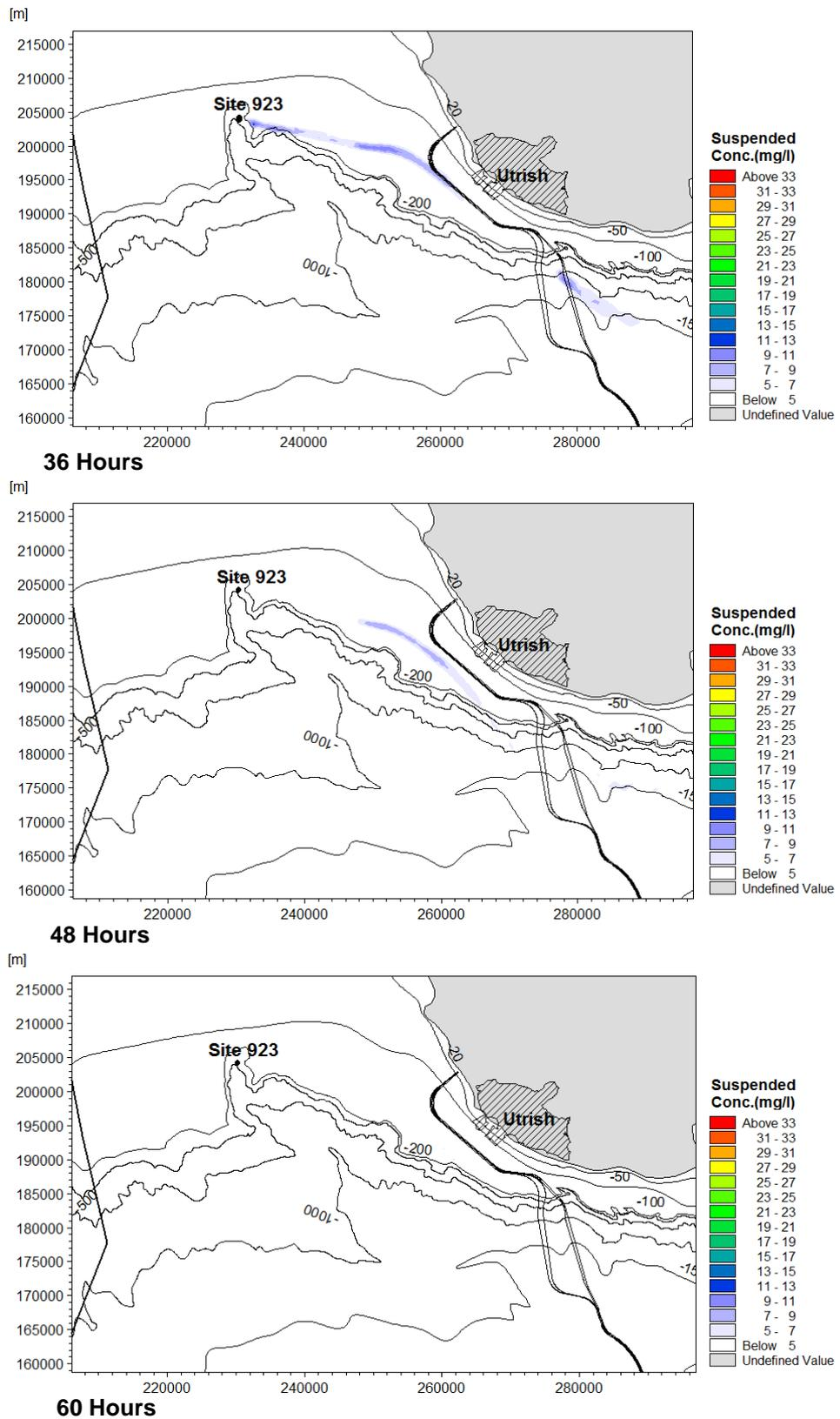
**Figure 3-9b Plume Development under Clockwise Currents (Scenario 3)**
