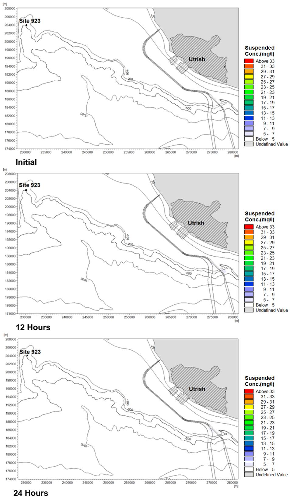
**Figure 3-19a Plume Development under Clockwise Currents (Scenario 5)**
