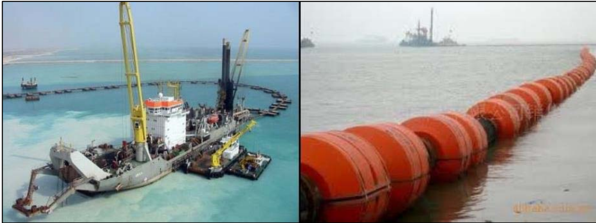
Figure 1.17: Cutter Suction Dredger with Floating Hose
