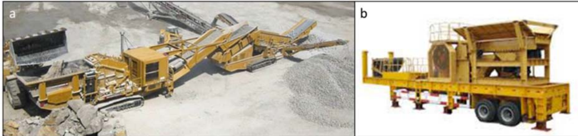
Figure 1.10: Typical mobile stone crushers (large diameter (a), small diameter (b))
