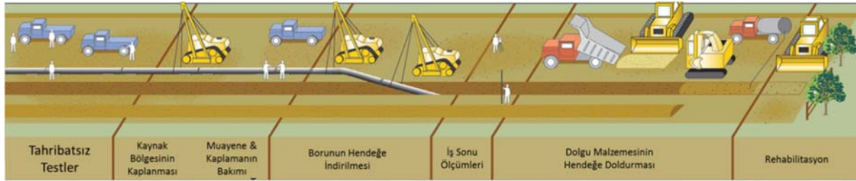
Figure 14.5: Phases of Typical Land Construction Technique for Pipelines
