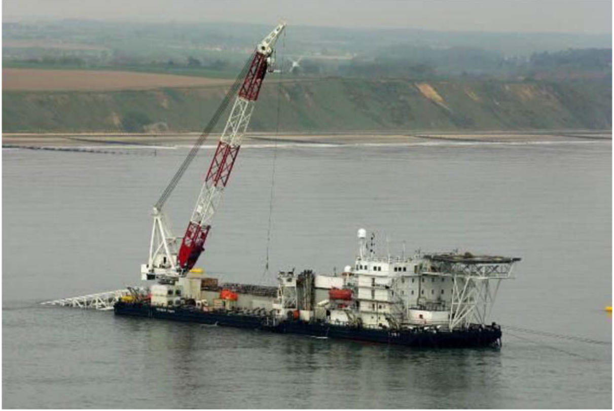
Figure 14.4: S-Lay Pipe-laying Vessel
