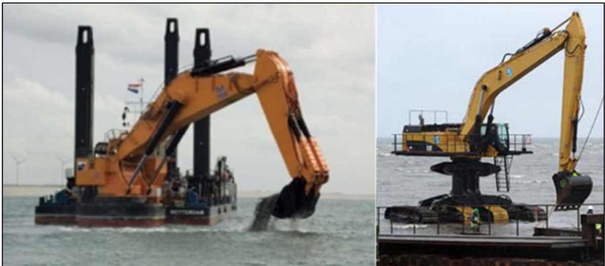
Figure 1.20: Backhoe Dredger on a Self-Elevating Pontoon (Left) and an Elevated Excavator (Right)
