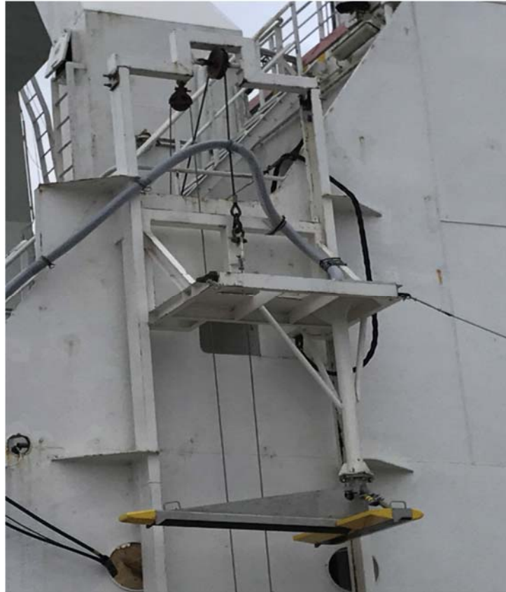
Figure 6.288: Satellite Complex of the Echo-Sounder
