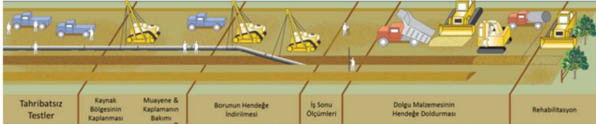
Figure 1.25: Phases of Typical Land Construction Technique for Pipelines
