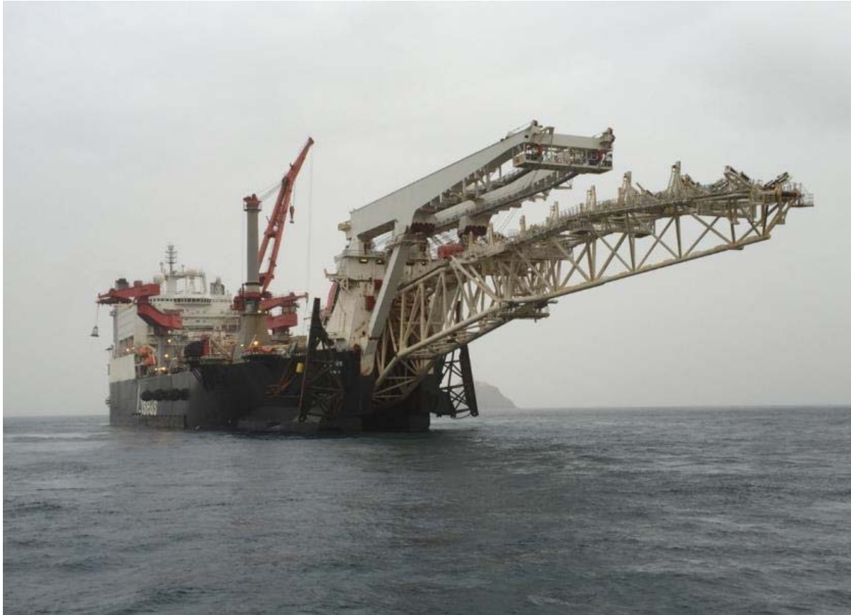
Figure 1.12: Typical Deep Water S-Lay Vessel (Image supplied courtesy of 'Allseas, Switzerland')
