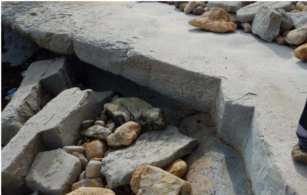
Figure 6.74: Medium Competent, Carbonated, Fine Stratified Mudstone with Joint Systems from Soğucak Formation
