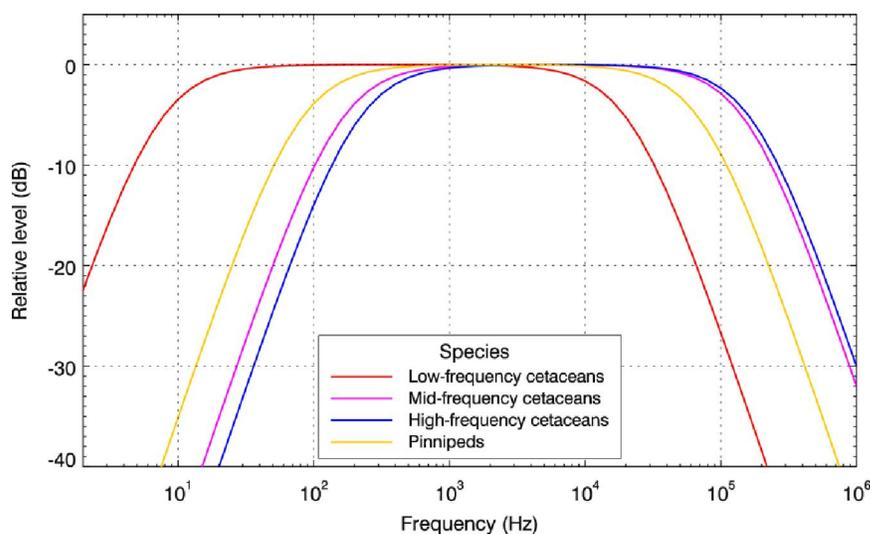
Figure 2. The standard M-weighting functions for the four underwater functional marine mammal hearing groups (Southall et al. 2007).
