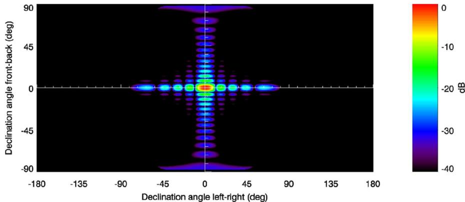
Figure 8. Calculated beam pattern for a rectangular transducer with a  $4^\circ \times 10^\circ$  beamwidth. The beam power function is shown relative to the on-axis level using the Robinson projection.
