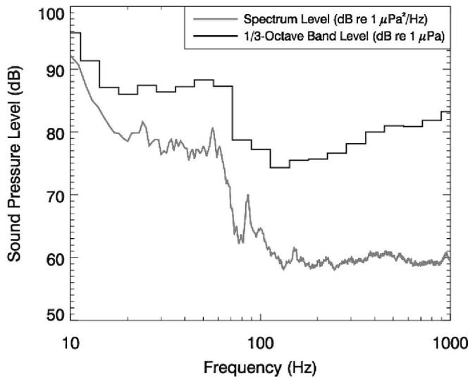
Figure 1. Ambient noise power spectrum (grey line) and the corresponding 1/3-octave-band levels (black line), plotted on a logarithmic frequency scale.
