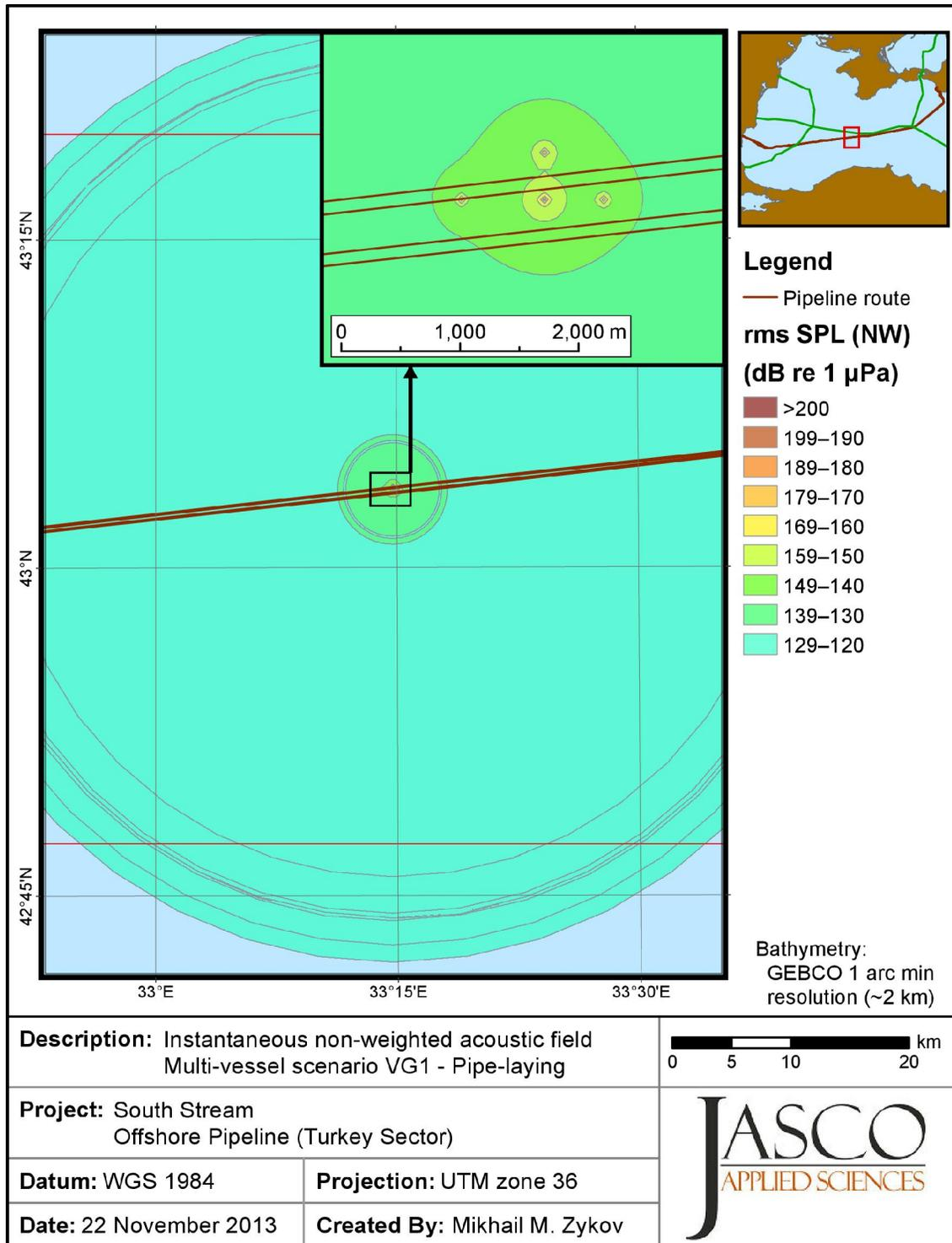
Figure 18. Broadband (10 Hz–20 kHz) maximum-over-depth sound pressure levels for the pipe-laying vessel group (VG1). Blue contours indicate water depth in metres.
