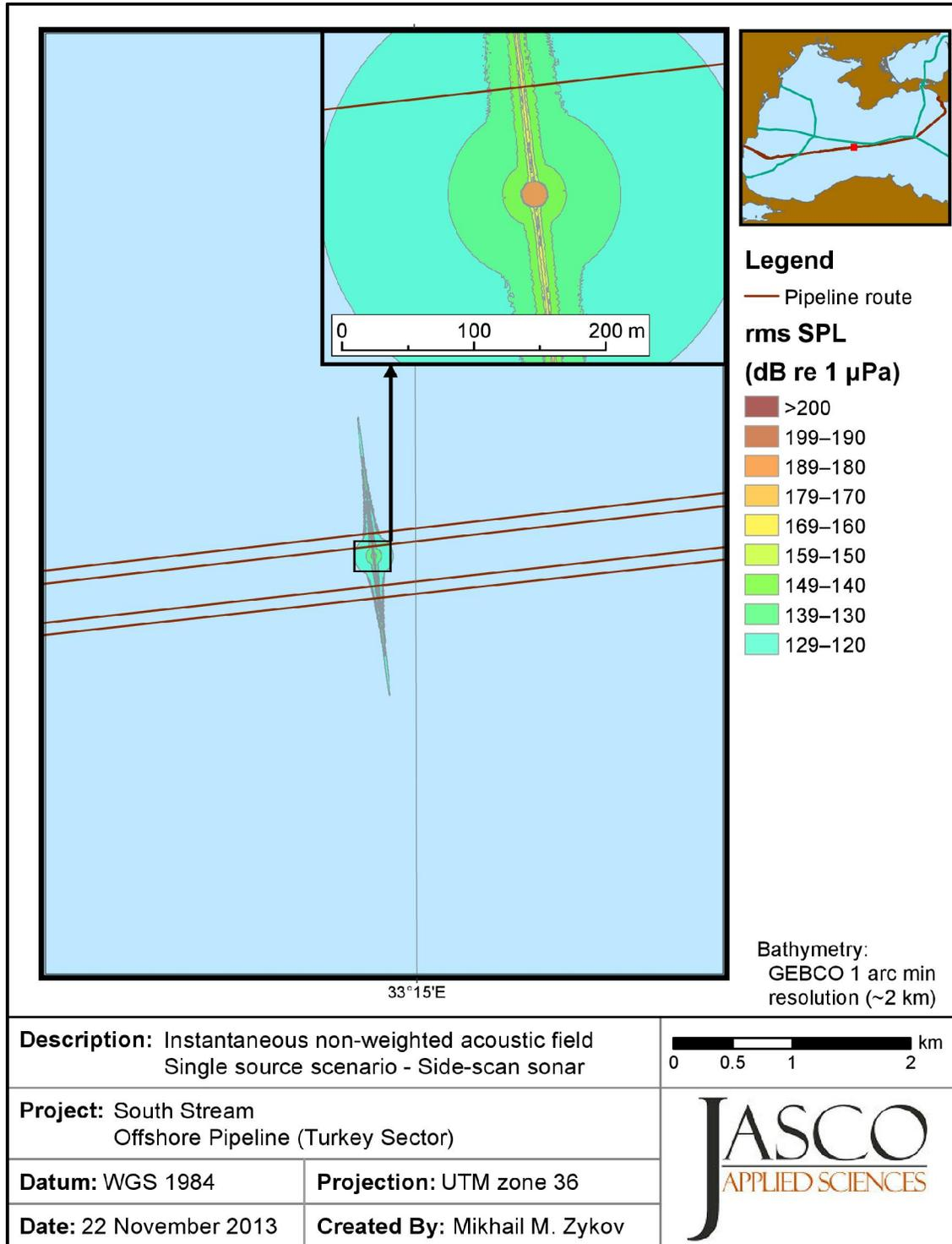
Figure 17. Narrowband (1 Hz at 75 kHz) maximum-over-depth sound pressure levels for the Edgetech Full Spectrum Chirp side-scan sonar at the target site. Blue contours indicate water depth in metres.
