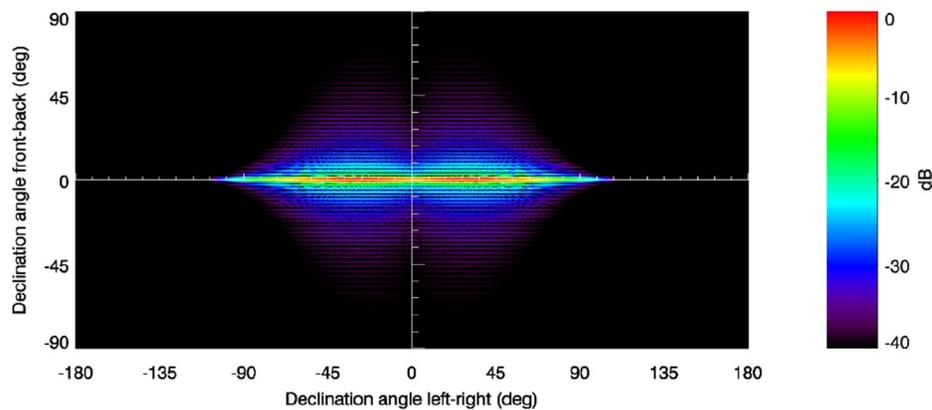
Figure 9. Calculated beam pattern for two rectangular transducers engaged simultaneously, with individual beamwidths of  $1.5^{\circ} \times 50^{\circ}$ , and a declination angle of  $25^{\circ}$ . The beam power function is shown relative to the on-axis level using the Robinson projection.
