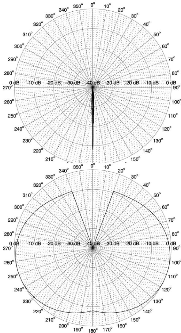
Figure 10. Vertical beam pattern calculated for the Edgetech Full Chirp Side-scan Sonar with two beams  $70^\circ \times 0.8^\circ$  width in the (left) along- and (right) across-track directions.
