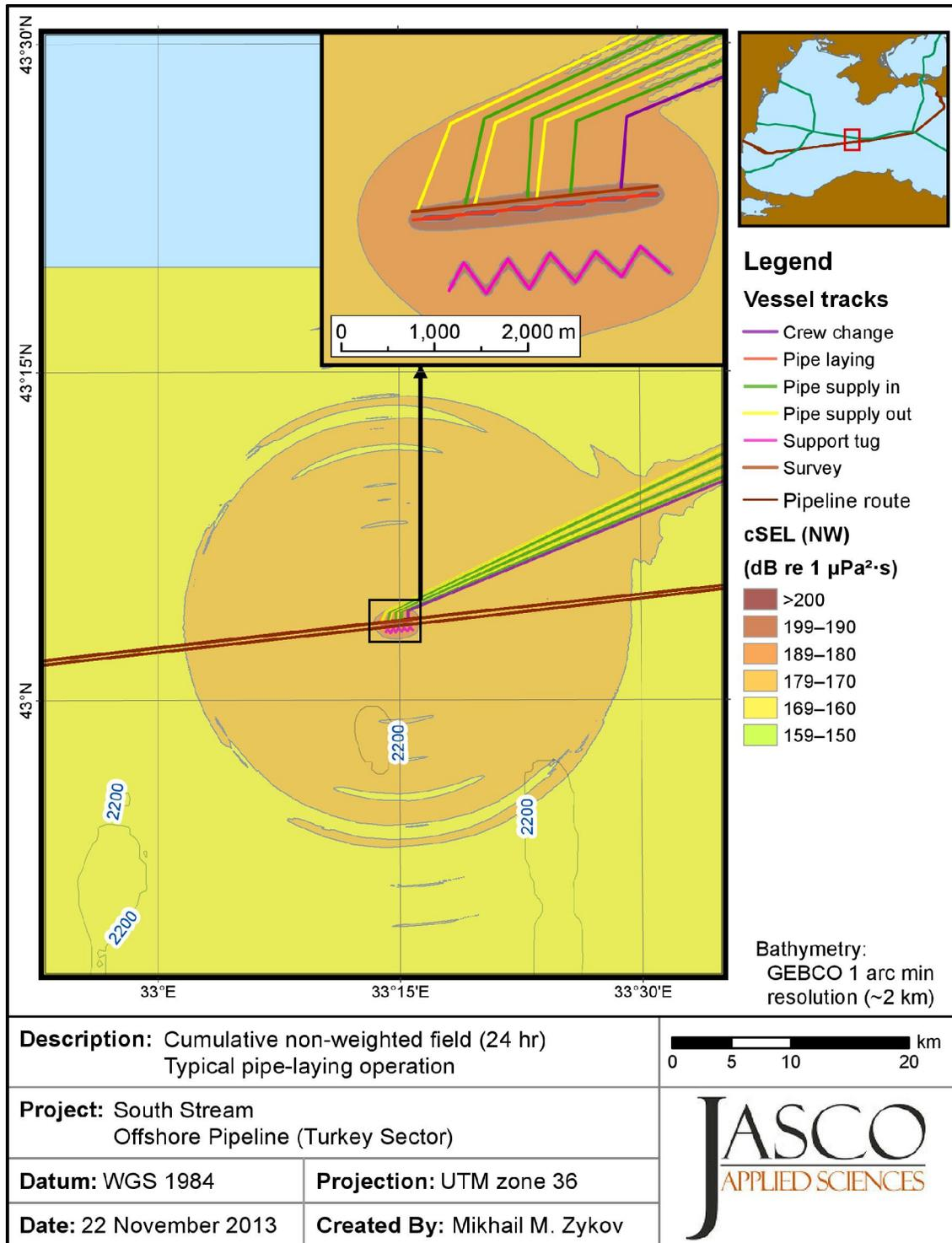
Figure 19. Colour-shaded zones depict broadband (10 Hz–20 kHz) unweighted cumulative SEL for the deep water pipe-laying scenario. The acoustic field is modelled for conditions prevalent in February. Blue contours indicate water depth in metres.
