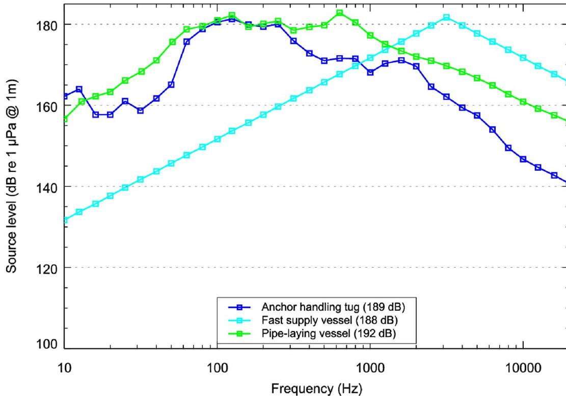
Figure 5. Source levels for the modelled vessels in 1/3-octave-bands. The numbers in the brackets indicate the broadband level in dB re 1 µPa at 1 m (rms SPL).
