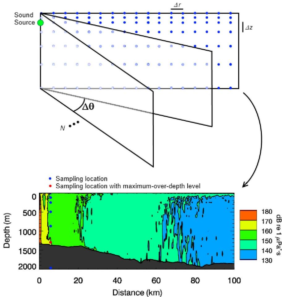
Figure 11. The  $N \times 2$ -D and maximum-over-depth modelling approach used by MONM.
