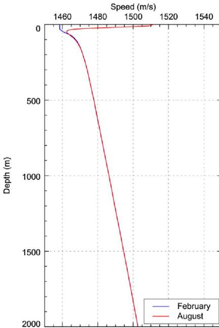
Figure 13. Comparison of sound speed profiles for February and August at the modelled site, derived from data obtained from *GDEM V 3.0* (Teague et al. 1990, Carnes 2009).
