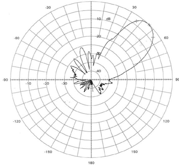
Figure 7. Vertical cross section of a beam pattern measured in situ from a transducer used by Kongsberg (source: pers. comm. with the manufacturer).
