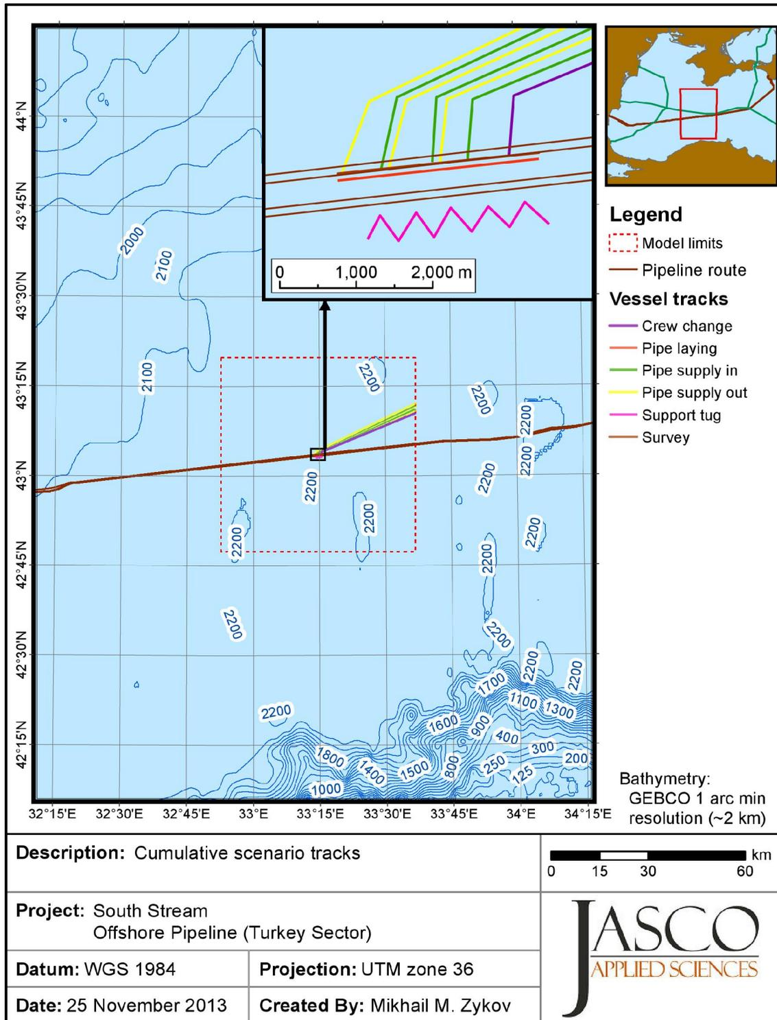
Figure 14. Tracks geometry for cumulative exposure modelling scenario.
