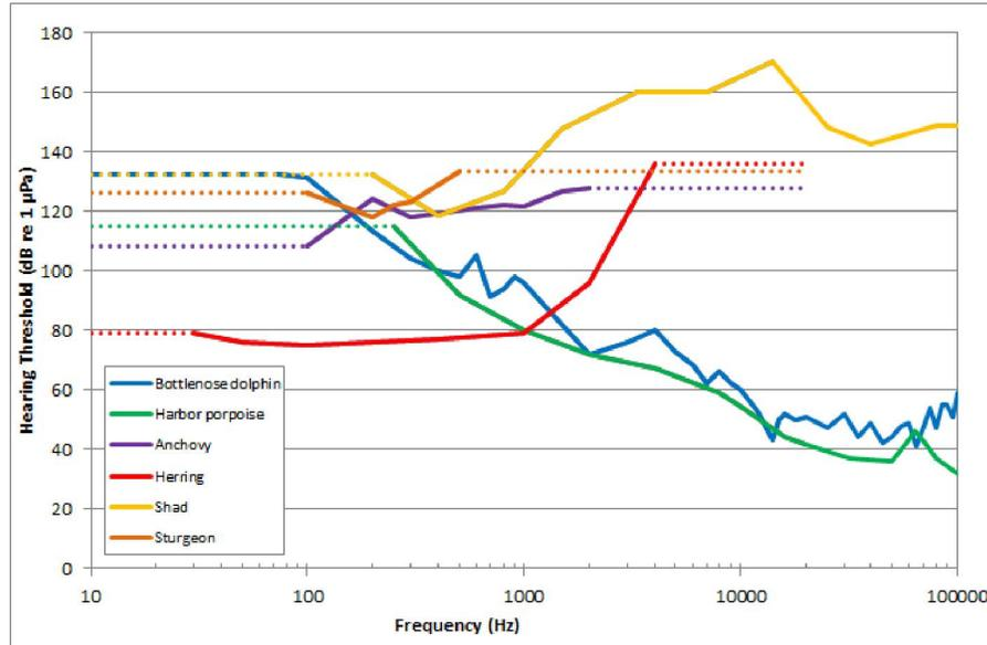
Figure 4. One-third-octave-band audiograms for bottlenose dolphin, harbor porpoise, anchovy, herring, shad, and sturgeon . Dotted lines represent extended hearing thresholds for modelling purposes.
