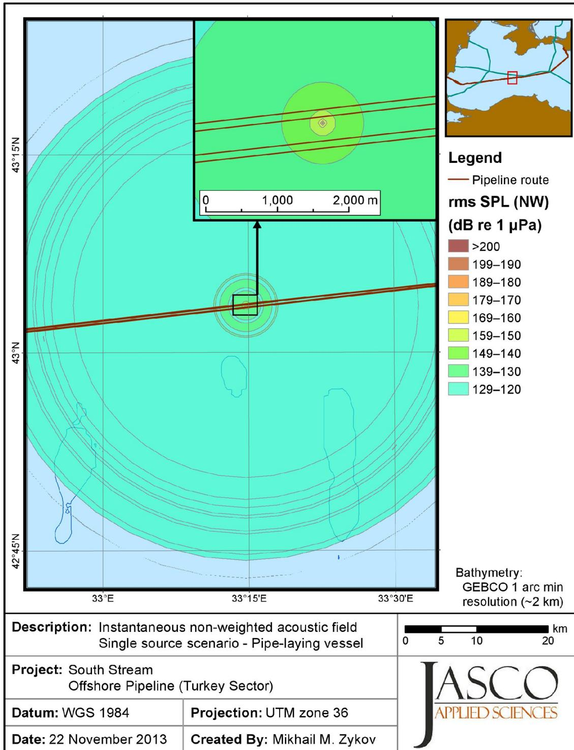
Figure 15. Broadband (10 Hz–20 kHz) maximum-over-depth sound pressure levels for the pipe-laying vessel at the target site. Blue contours indicate water depth in metres.
