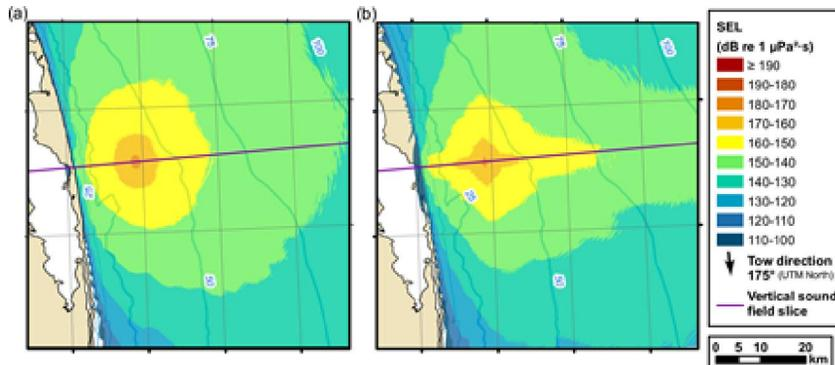
Figure 12. Maximum-over-depth sound exposure level (SEL) colour contour maps for two arbitrary sources.
